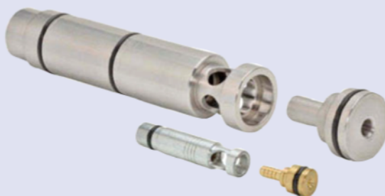
Top: Custom made C350H-303 stainless steel venturi cartridge 5.375" L x 1" dia. Bottom: Standard Mid Series C150H aluminum/brass cartridge is 2.2" L x 0.40" dia. Both cartridges generate up to 28"Hg.
