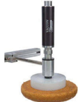
Remove cakes from a conveyor and place in box without damage
