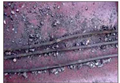
WSOR cables covered and undamaged by weld slags
