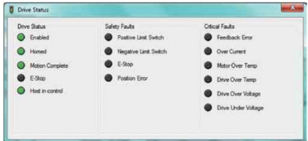
Figure 13-23: Drive Status tool indicates Software (Host) is in control.
