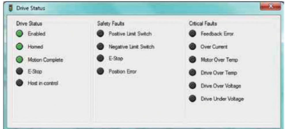
Figure 13-25: Drive Status tool indicates EtherNet/IP (or Modbus TCP, Modbus RTU) is in control.
