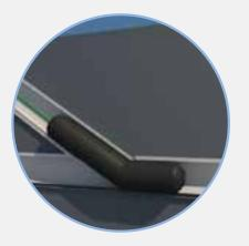
IN THE SECOND PHASE, THE REMAINING PART OF THE PLUG IS INFLATED TO COMPLETELY STOP THE FLOW
