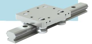
**IVTAAW** linear guides offer an alternative and more cost-effective solution to profile rail systems. Composed of a precision machined aluminum anodized rail with embedded hardened steel races, the IVTAAW linear guide is lightweight without sacrificing strength.
