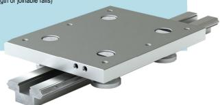
**IVTAAE** linear guides provide a double wide base rail option for the IVT family that can easily integrate a variety of drive options. Composed of a precision machined aluminum anodized rail with embedded hardened steel races, the IVTAAE linear guide is lightweight without sacrificing strength.
