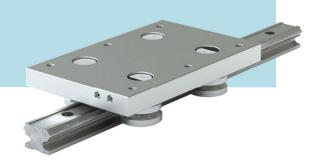
**IVTAAB** linear guides provide a wider base rail option for the IVT family that can easily integrate a variety of drive options. Composed of a precision machined aluminum anodized rail with embedded hardened steel races, the IVTAAB linear guide is lightweight without sacrificing strength.
