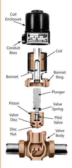
**MAGNATROL SOLENOID OPERATED VALVES** are used to control the flow of liquids or gases, generally in conjunction with automatic control apparatus such as thermostat, float switch, time switch, or flow meter.
