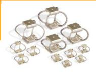
Smaller than traditional Wire Rope Isolators, these unique products provide simultaneous shock and vibration attenuation where sway and package space are a premium. Their symmetrical design provides consistent, multi-axis isolation and their small size permits isolation of individual system components, rather than the entire system. This creates a cost-effective shock and vibration solution.
