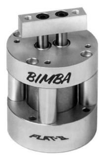
Flat-II nonrotating, double-acting cylinder provides the answer to applications where rotation cannot be tolerated and space is at a minimum. Nonrotation is achieved with dual piston rods and a rod end block that insures the rods work in tandem. Flat-II eliminates the need for external alignment devices, such as guides, rods and alignment posts or pins.
